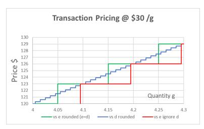
If the user must have a scale with e = d, then it forces them to go to 0.01 g e to service loads at the 1 g level. For that scale 50 e is 0.5 g, and the 1 g loads weighed are near 100 e. Precision scales rarely use 2 or 5 divisions, so capacities get reduced by a factor of 10 to move down to the next smaller division size. Blocking the use of e=10d may force many users to purchase two scales where a single scale would have been suitable if using a scale with a differentiated d were not blocked.
