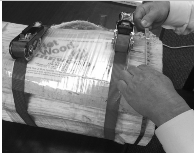
Figure 13. Strapping the End of a Bundle
