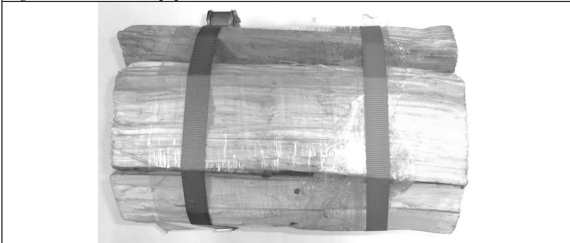
Figure 7. Bundle with Straps placed 10 cm (4 in)
