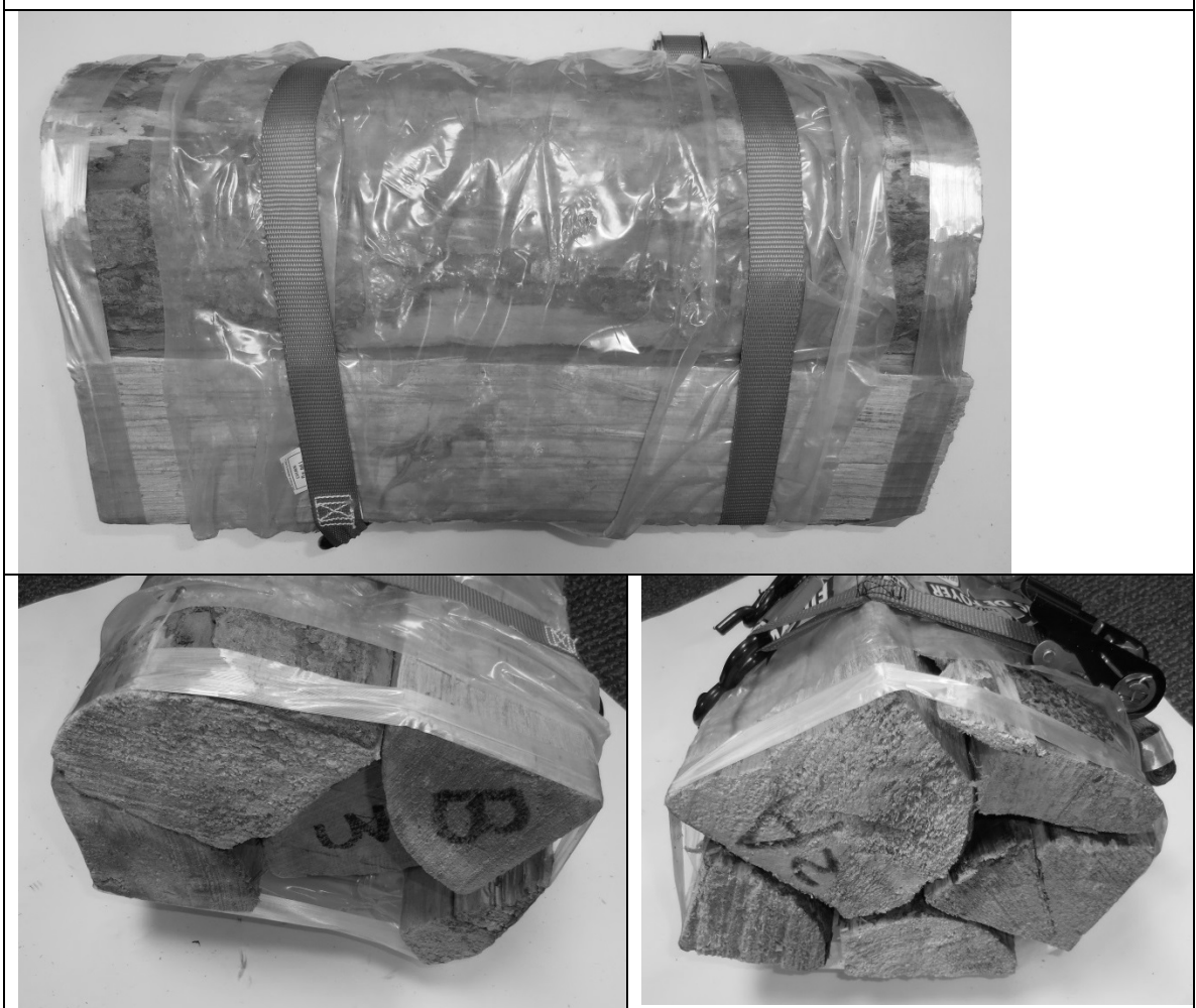
Figure 8. Bundles with Fiber Reinforced Packing Tape around the Perimeter of the Ends
