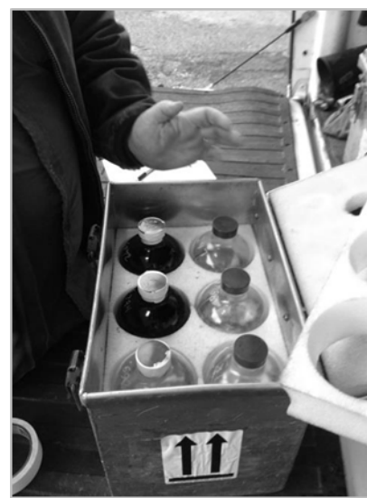
Figure 13b. Sample Box Showing Insulation.
