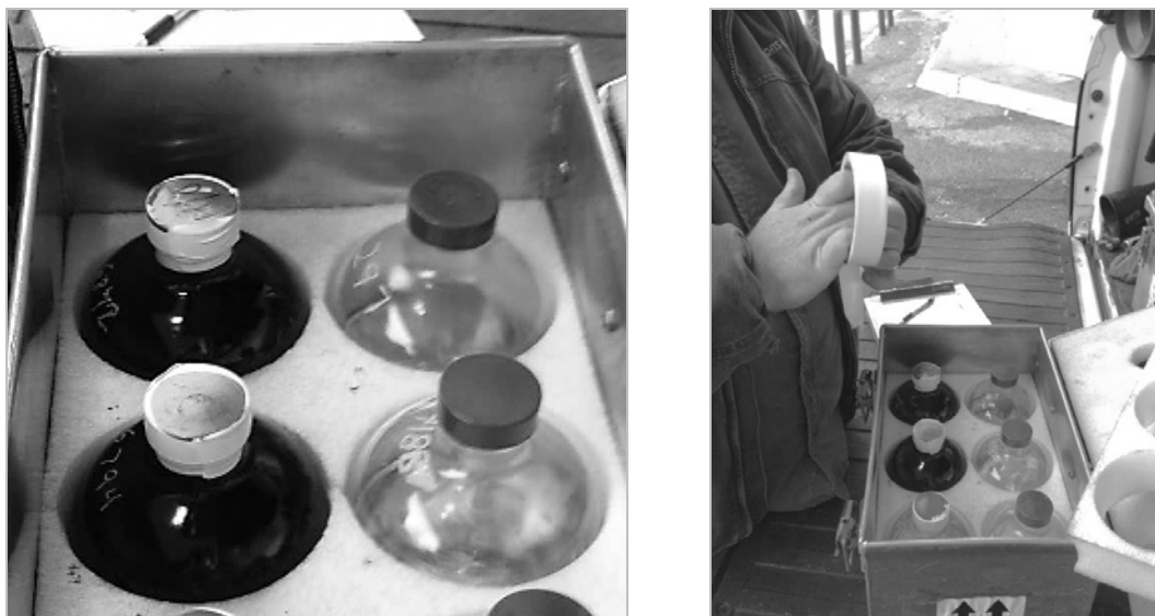
Figure 19. Sealing Tape Applied to Amber Sample Bottles
