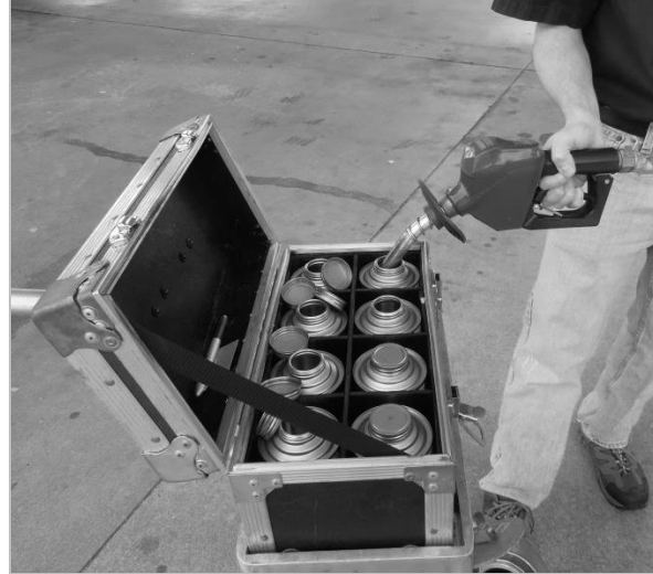
18. Fuel Sampling Cart with Sample Container bonded to cart and ground.*
